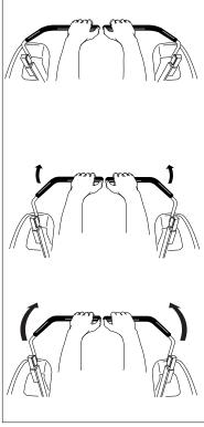
Figure 4. Move Control Levers Gradually
